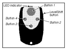
control. But instead of putting 12 buttons on the remote, we made it easy: First, the button you use the most — button 1 to arm, disarm, lock and unlock — is larger than the others. Buttons 2, 3 and 4 are the smaller buttons to the right, below and left of button 1. The *LevelShift* button on the side of the remote control allows you to select channels 5–12:
